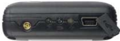
GPS Antenna Interface
